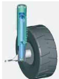
Cylinder for the loader suspension system
