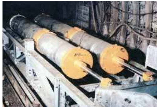
Cylinders for pneumatic belt tension
