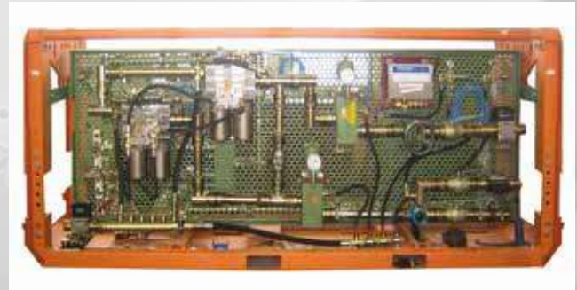
High pressure filter station for filtration of longwall hydraulics or spray water
