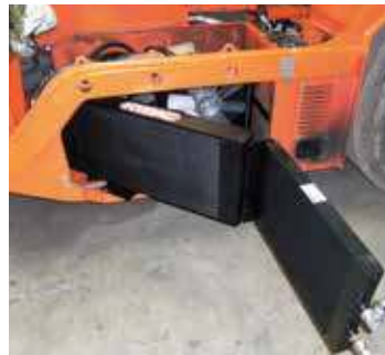
Combination cooler for drive motor cooling
