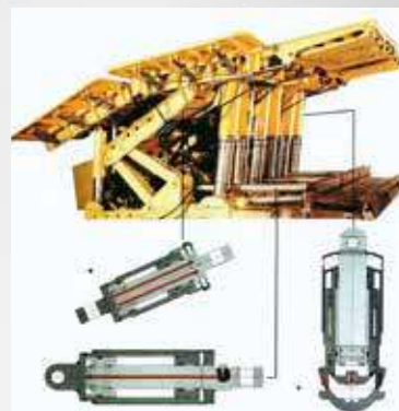
Sign. Cylinder for pressures up to 1,500 bar
