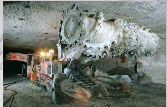
Room-and-pillar extension with Continuous Miner
