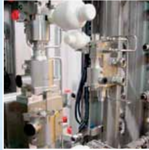
Diaphragm Accumulators used for pulsation dampening during valve actuation. Vol. 0.075 l up to 4 l. Pressure up to 15,000 psi (1030 bar)
