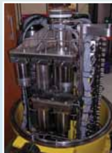
Stainless Steel Filters in subsea modules.
