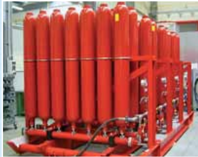
Bladder Accumulator Rack on HPU. Customer-specific engineering and computer-based simulation.
