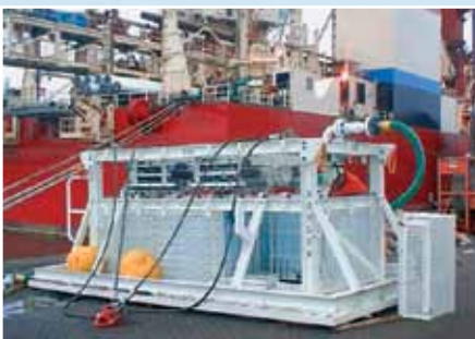
Seawater filtration with disposable custom designed Filter Elements for pipeline flooding.
