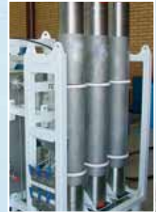
Stainless Steel Piston Accumulator Station used on HPU.
