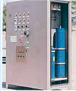
Accumulators up to 15,000 psi (1030 bar) and/or Filters to actuate valves in Well Head Control Panel.
