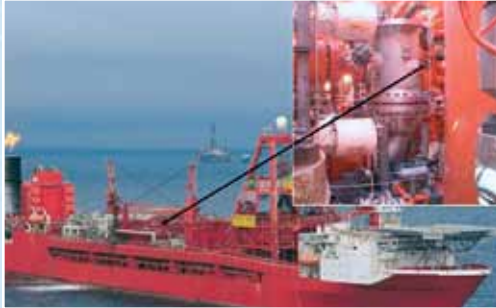
Floating Production Storage and Off-loading (FPSO). Improving the cleanliness of PRODUCED WATER before disposal at sea using Automatic Backflush Filters AutoFilt® RF3 (flow rate 800m 3 /h).
