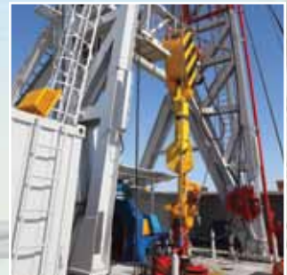
Power Swivel powered and controlled by HPU.
