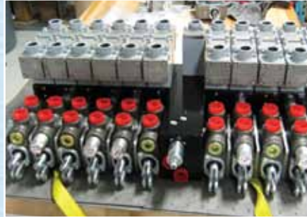
Sectional Spool Valve Control Block with ATEX approved Solenoids .
