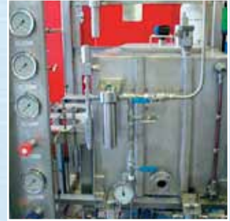
High Pressure Stainless Steel Filters - HPSSF on HPU unit. Up to 10,000 psi (690 bar)
