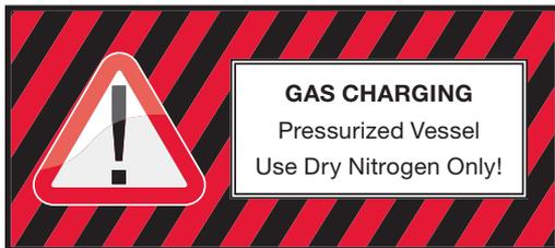
Hydraulic accumulators are pressurized vessels and only qualified technicians should perform repairs. Never weld, braze, or perform any type of mechanical work on the accumulator shell. Never lift the accumulator by the gas valve. Always drain the fluid completely from the accumulator before performing any work, such as recommended repairs (*see Maintenance Instructions in Accumulator Catalog #02068195*) or connecting pressure gauges.
