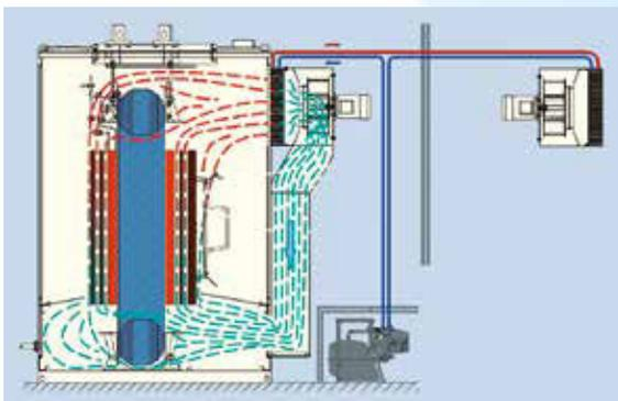
**Dry transformer:** separation internal / external air by 2 Water / Air Coolers and a Water-Glycol Circulation.
