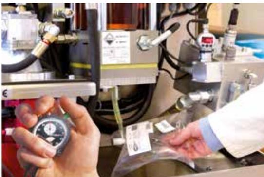
Simple gas discharge to determine the gas formation rate.
